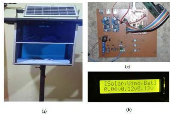
Fig. 3: (a) Physical appearance; (b) Final PCB; (c) LED Display
